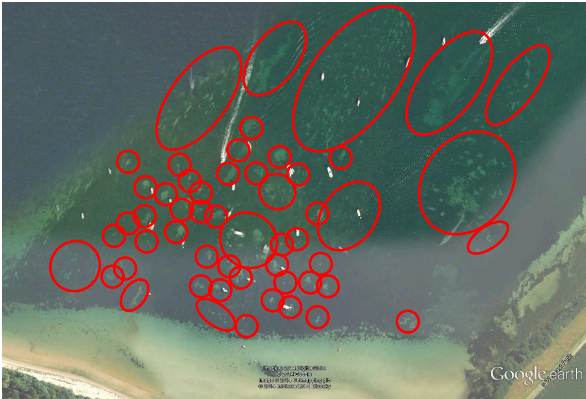
Figure 3. All red circles represent holes created by anchor damage or mooring chains in the seagrass, as ground truthed by Seahorse Trust divers and others such as National Oceanography Centre (NOC) divers under the supervision of Dr Ken Collins. (Courtesy of Google Earth, image 2009)
